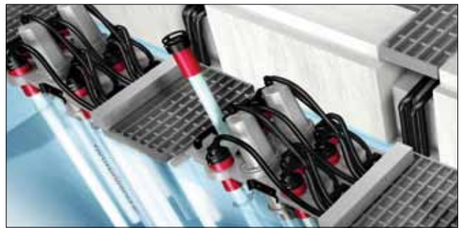
The lamps and sleeves can be easily removed by a single operator. A safety electrical disconnect in the lamp plug prevents the removal of an energized lamp from the sleeve.
